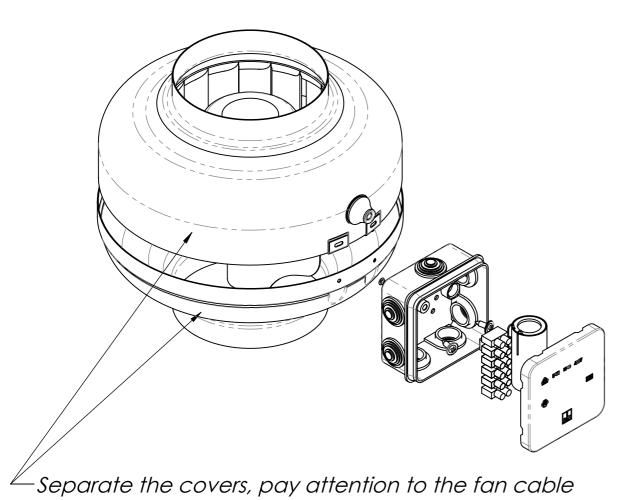
Remove 4 screws holding fan impeller, take fan impeller out. Make sure to mind the cable.
