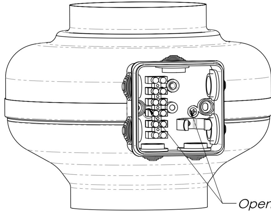
*Open/disassemble the box, remove 2 screws*
